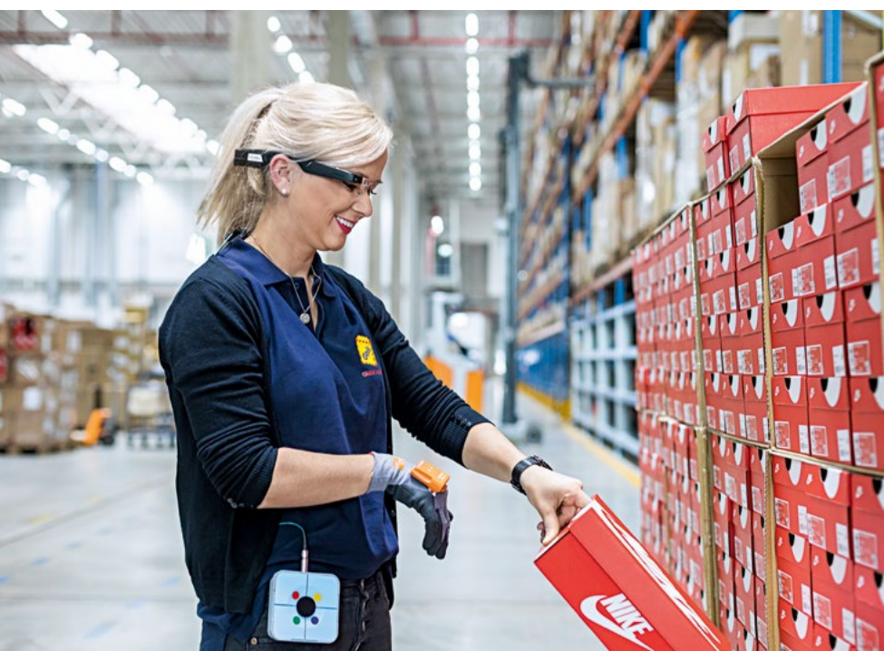
A clever combination: Google Glass and picking glove with built-in scanner.
